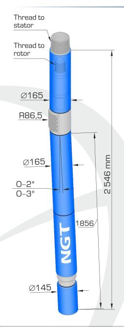
Bearing section S–165.NGT.M1 is a new short bearing section featuring enhanced operation life.
