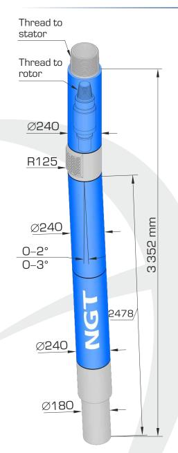
Bearing section S–240.NGT.M1 is a new short bearing section featuring enhanced operation life. The bearing section is used in PDM power sections of 240 mm diameter and for drilling oil and gas wells with 295.3-444.5 mm rock and PDC bits.
