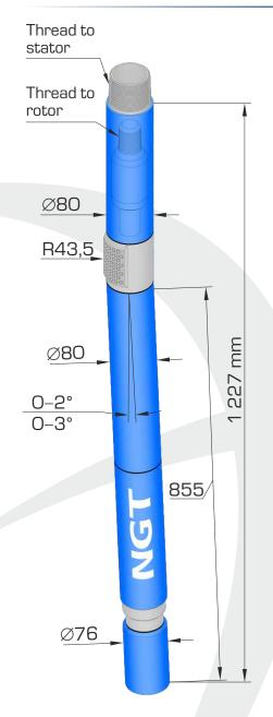
Bearing section S-76.NGT.M2 is a new short bearing section featuring enhanced operation life.
