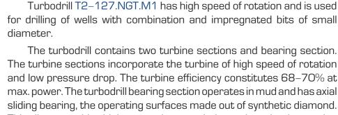
The turbine sections incorporate the turbine of high speed of rotation and low pressure drop. The turbine efficiency constitutes 68-70% at max. power. The turbodrill bearing section operates in mud and has axial sliding bearing, the operating surfaces made out of synthetic diamond. This allows reaching high power characteristics and overhaul operation
