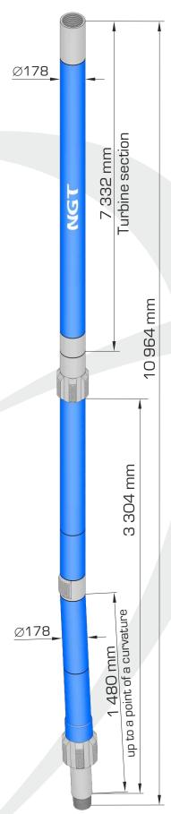
Turbodrills TBS1–178.NGT.M1 and TBS1–178.NGT.M2 are new universal turbodrill–whipstocks with an ultra–short arm to the point of axes curvature.
