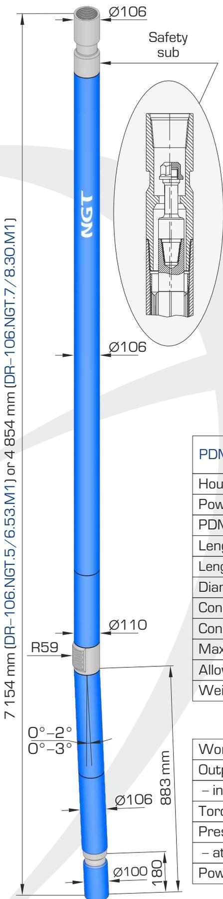
PDM's DR-106.NGT.5/6.53.M1 and DR-106.NGT.7/8.30.M1 are new universal hydraulic downhole motors used for:
